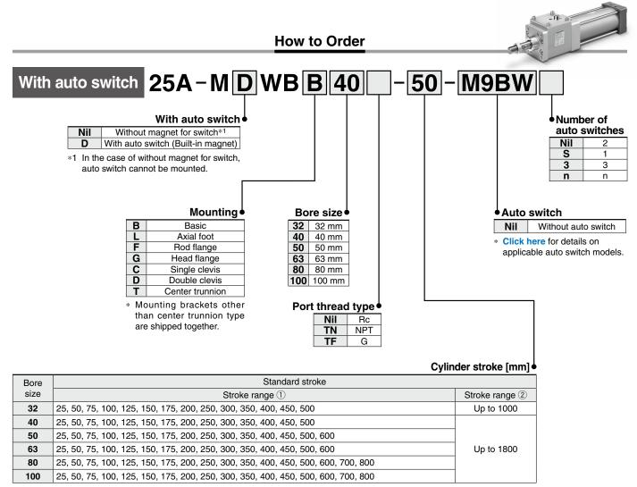
The manufacturing of intermediate strokes is possible. (Spacers are not used.)
