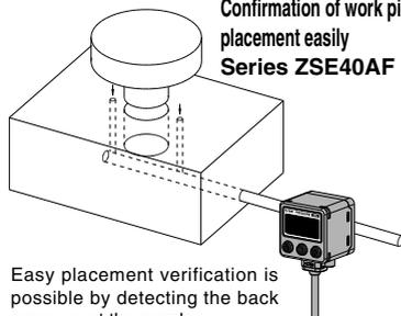
Easy placement verification is possible by detecting the back pressure at the nozzle.
