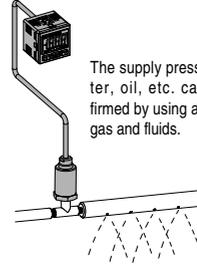
The supply pressure of water, oil, etc. can be confirmed by using a sensor for gas and fluids.
