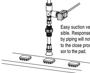
Easy suction verification is possible. Response delays, caused by piping will not be a factor, due to the close proximity of the sensor to the pad.
