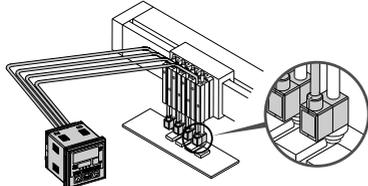
Due to the small size, the sensor can be installed close to a pad.
