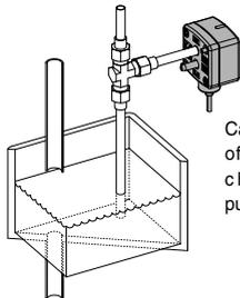
Can detect the level of a liquid through changes in the purge pressure.
