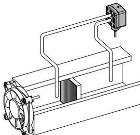
The filtration and replacement periods can be controlled by monitoring the clogging of the filter.
