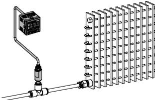
A low pressure sensor (PSE532-□) is used to detect minute differences. The auto shift function reduces the influence of fluctuations in the supply pressure.
