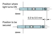
To set the detection point of the second point (and subsequent points), you will be required to prepare a new switch and set it from step 1.
