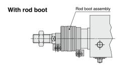
\* Replaceable with the rod boot assembly For details on replacement part numbers, refer to page 245.
